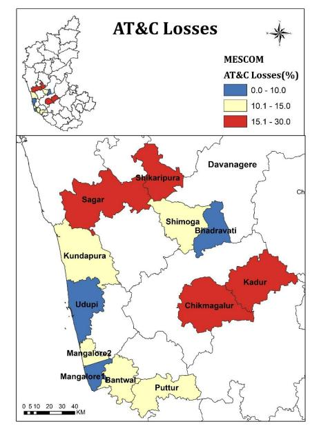
Figure 4: Division-wise AT&C loss heat map for MESCOM in FY16
