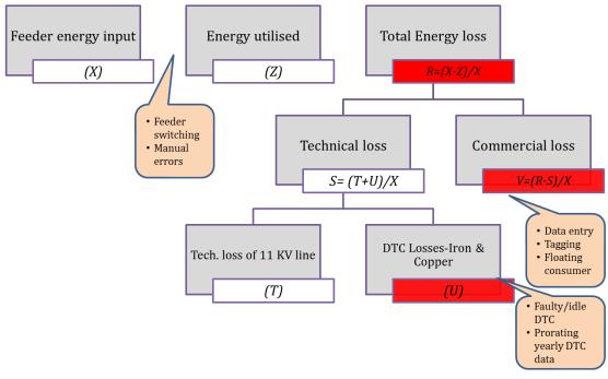
Figure 10: Feeder-level analysis for a sample feeder based on DISCOM data
