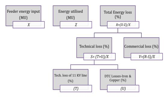
Figure 9: Schematic representation of 11kV-feeder-level analysis
